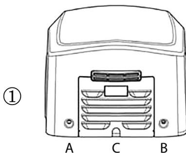
To remove the front cover, place the unit in front of you and pull it towards you by exerting slight pressure on the sides as shown in the following figure:
